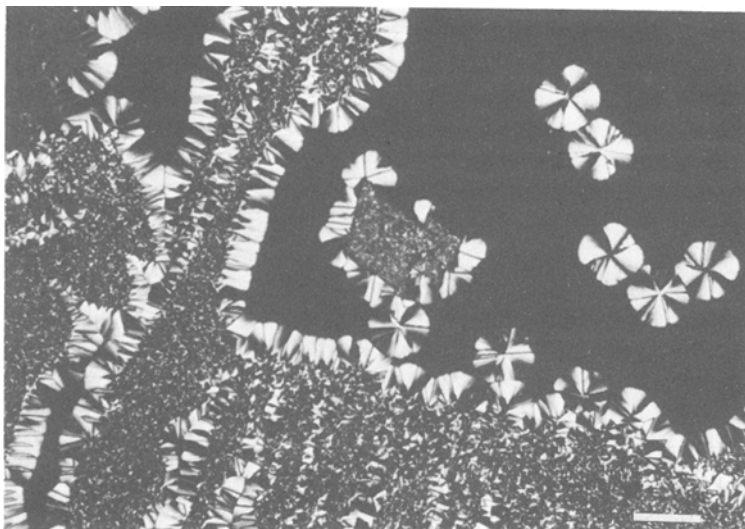
Figure 1 Selenium film crystallized by heating to T_c = 180^\circ\text{C} from the glassy state in the presence of p -terphenyl crystals (lower part). Crystallization has been arrested by quenching back to room temperature. Optical micrograph with crossed polarizers; scale bar: 50\ \mu\text{m} .
